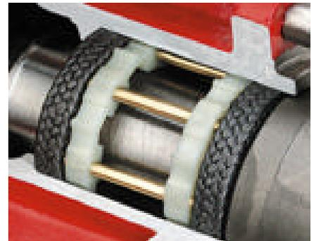
The idea to inject a soft, malleable and fibrous packing compound into the stuffing box, instead of using relatively hard braided packing rings, is not a new one. However, due to various reasons it has not been successful and this system has never become popular.
