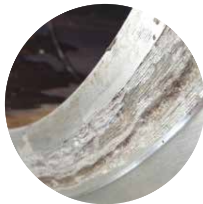
Corrosion caused by use of conventional graphite gaskets
