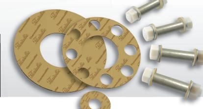
The Flexitallic I-Flex Fire-Safe Flange Insulating Set (FS-HP) is comprised of a fire safe insulating gasket, insulating sleeves, insulating washers and metal backing washers.
