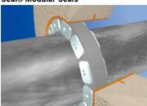
Century-Line® Model CS Sleeves are ideal for poured wall construction. Made of HDP1 thermoplastic, they are lightweight and easy to handle. Molded in waterstop and reinforcing ribs serve to anchor the sleeve in the wall and resist pour forces. Nailer end caps are provided to make placement in forms simple and accurate. Sleeves are available in 16 diameters, up to 25", and any length. In the event of a field change they can be shortened with ordinary hand tools.
