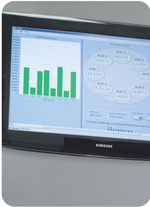
Real time visualisation of bolt loading to aid learning.
